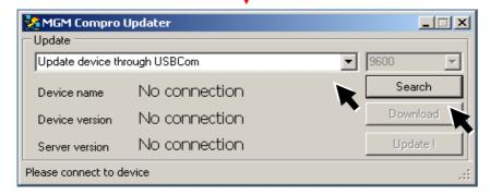
Plug the USBCOM++ module into the USB connector on your PC and if updating SW in controller connect also it using CC\_03 (without power supply yet) and press "Search" button.
