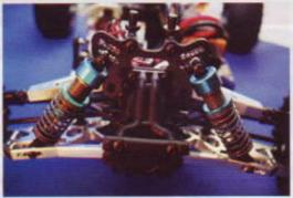
Tamiya TRF aluminum shocks fit well, but I swapped the lower ball ends for the stock CRTs. The Xtreme RC shock tower is made of super-strong carbon fiber and offers more mounting holes than I will ever need.
