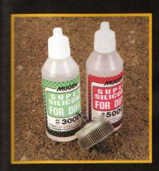
1/8-scale vehicles use sealed gear diffs, and different viscosity oils are used to tune the diff action. Dave applied this to the Slash, but because the stock diff wasn't a sealed type, he figured out how to seal it up using o-rings and some RTV silicone.
