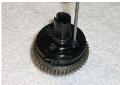
22) Install small cover assembly with 8mm flathead screws. Use blue threadlock. "tip" –If you find the internal gear mesh to be tight on final assembly, remove the small cover and install an additional gasket(included).
