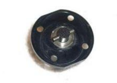
19) Put greased o-ring, washer, cross pin on outdrive shaft.
