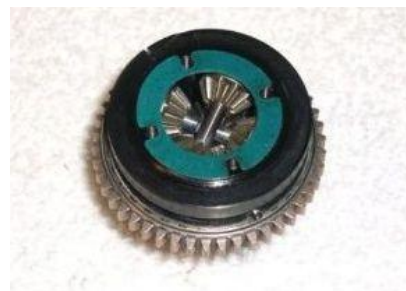
21) Fill diff cup with your choice of diff fluid. Fill just to top of gears. Place gasket on diff cup.
