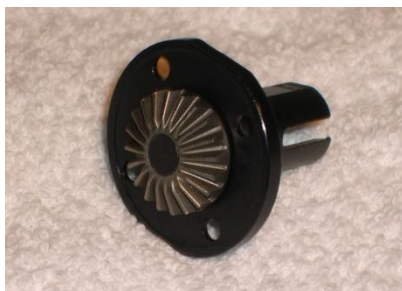
20) Put crown gear on outdrive shaft. "tip" – a dab of silicon fluid under the crown gear will help hold it in place during final assembly
