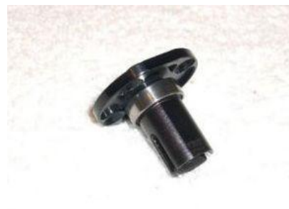
18) Install bearing and outdrive into small cover plate. Lightly grease the hole and/or outdrive shaft before assembly.
