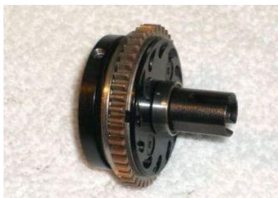
14) Put bearing on endplate and insert outdrive.
