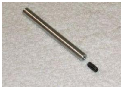
23) Put 4mm grub screw into adjustment tool until bottomed out. Use threadlock. – Set screw must be threaded into adjustment tool deep enough to allow the tool to "bottom out" on the adjustment ring in use
