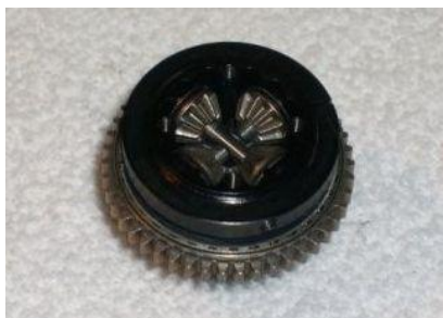
16) Install crown gear over outdrive shaft and cross pin. Install satellite gear assembly.
