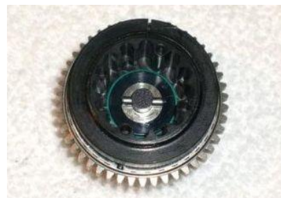
15) Put washer over outdrive shaft and insert cross pin thru cross hole.
