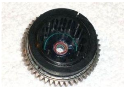
13) Put o-ring in groove. And lightly grease o-ring and outdrive hole.
